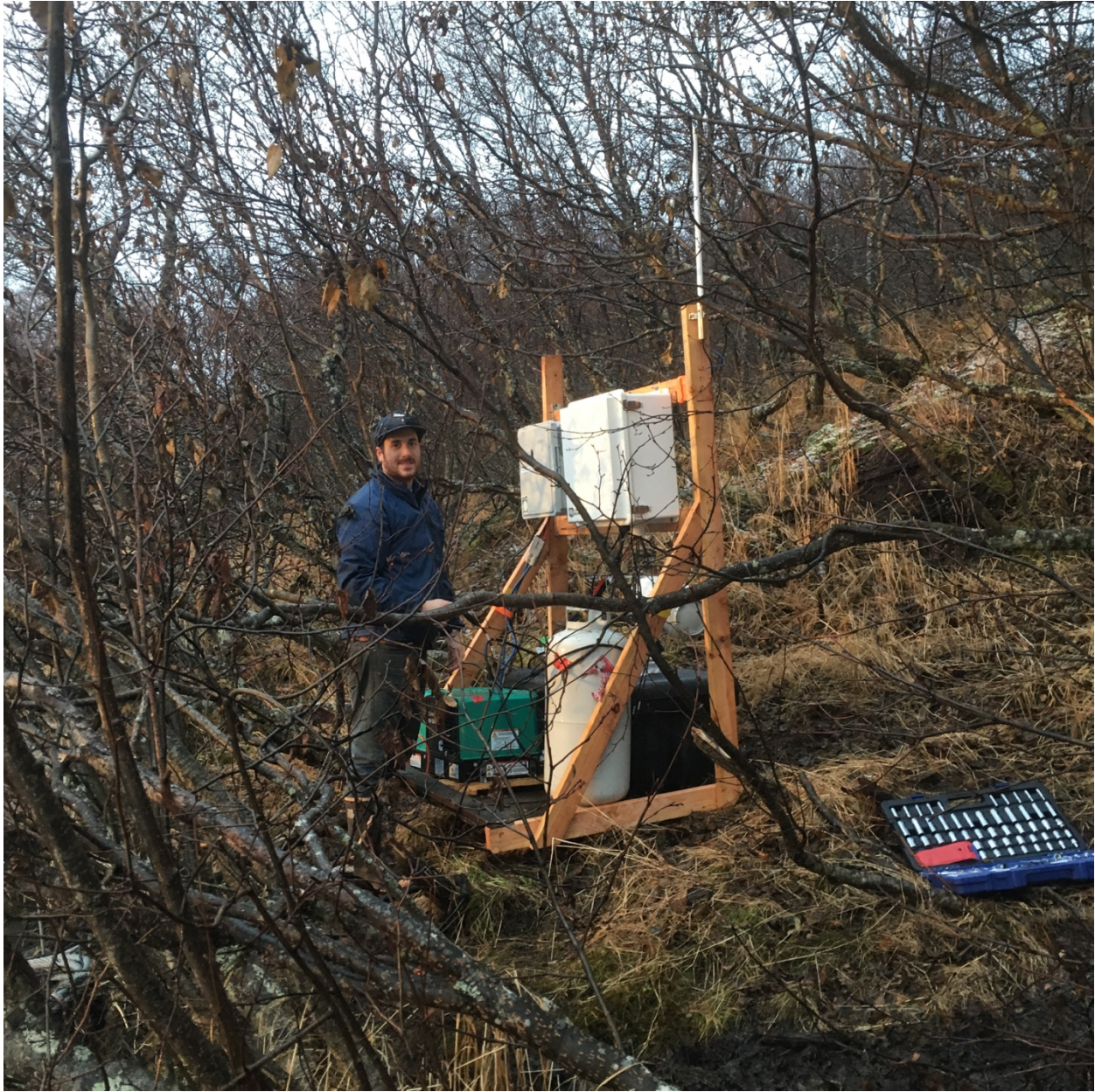
Figure 31. UAF personnel with the remote power/data telemetry river ice monitoring system on the bank of the Kvichak River, downstream of the Village of Igiugig, Alaska, November, 2016.
